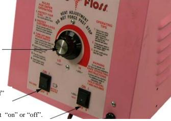
Main Switch: Turns motor "on" or "off" and supplies voltage to the heat switch.
